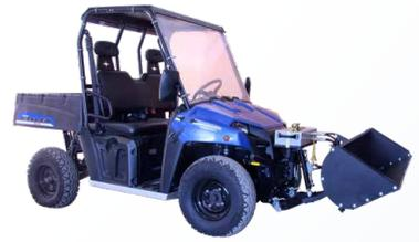
\* Hydraulic bucket 1500mm assembly requires a 1500mm wide UTV front-mount standard plow blade see page 18-19.
